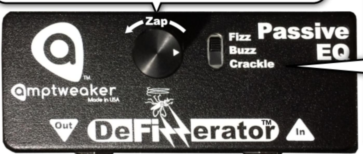
**Switch**—Chooses frequency of Zap control, Fizz is highest, Crackle lowest
