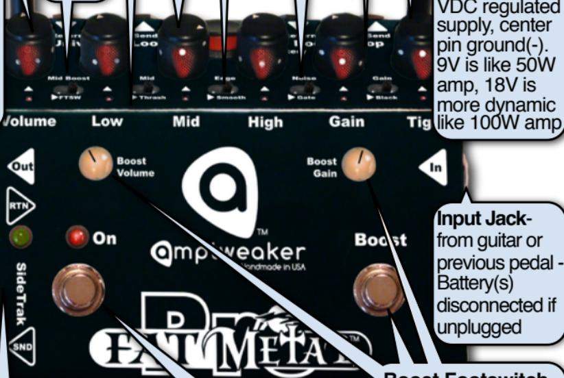
**SideTrak Loop**—This loop is active when the FM Pro is bypassed. Send to 'clean effects' In, Return from 'clean effects' Out.
