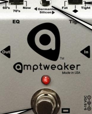
**DC Jack**—use regulated 9V–18VDC supply, with (-)center pin...9V is the most distorted, 18V is cleaner, and louder—is better for clean boosting
