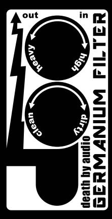
The **GERMANIUM FILTER** is a rich boost, overdrive, fuzz, vintage-izing pedal. The pedal uses a specially matched pair of obsolete 1960s Russian germanium transistors unconventionally to create a particularly full and saturated sound.
