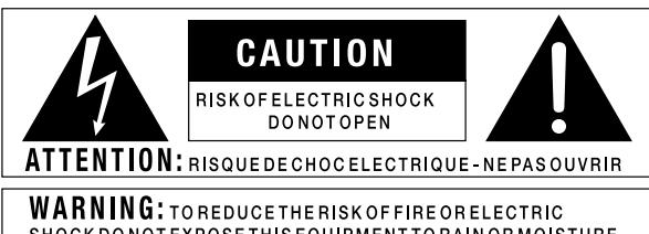
The symbols shown above are internationally accepted symbols that warn of potential hazards with electrical products. The lightning flash with arrowpoint in an equilateral triangle means that there are dangerous voltages present within the unit. The exclamation point in an equilateral triangle indicates that it is necessary for the user to refer to the owner's manual.
