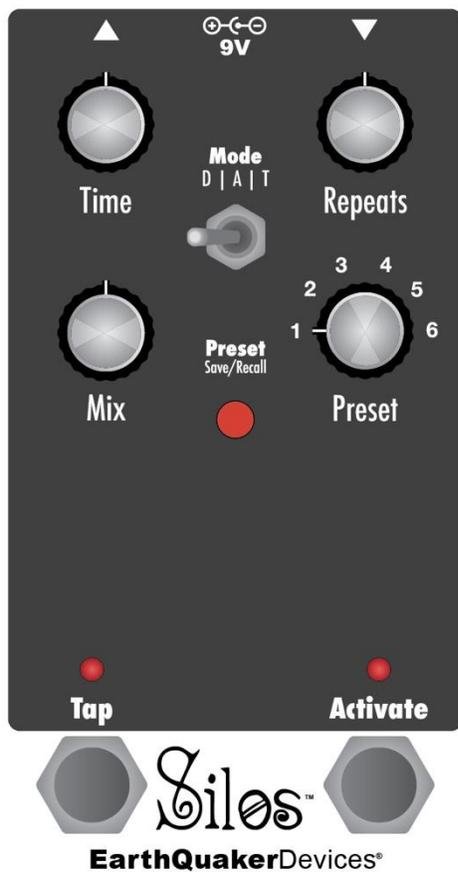
Commandes de la EarthQuaker Devices Silos
