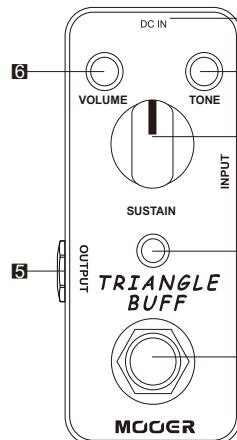
1. **TRUE BYPASS Footswitch:** Push down the footswitch to toggle between on and bypass status.
