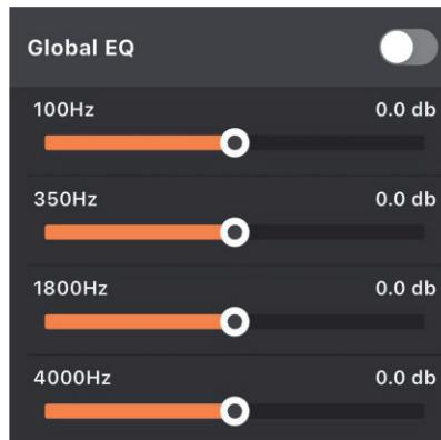
Global EQ applies EQ adjustments to the output of the M2, helping to minimize tonal changes caused by different sound reinforcement equipment.
