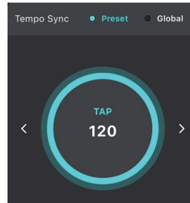
Click the icon to enter Tempo speed settings. You can choose the mode for Tempo Tap Tempo, either synchronizing the speed of preset effects (modulation and delay) or globally (preset effects and drum machine). You can set the speed by continuously tapping the circle area or use the left and right arrows for precise adjustments.
