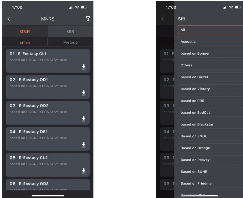
You can use this feature to download MNRS cabinet samples from the official section. Click on the GNR file and select the Entire cabinet sample (including the cabinet speaker) or Preamp (amp stage) sample, and use the filter icon in the top-right corner
