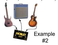
GROUND LOOP NOISE? Hooking two amps together via an ABY-G box can sometimes create a LOOP ANTENNA which causes hum (also known as Ground Loop Hum, 60Hz Hum or 60 Cycle Hum, 50Hz in Europe). This is not caused by the ABY-G but by the connection of two amp grounds via the ABY-G. If this does occur, it can be easily corrected. Visit www.morleyproducts.com for information on eliminating Ground Loop Hum & Noise with our Hum Exterminator or outside North America, the Hum Eliminator.
