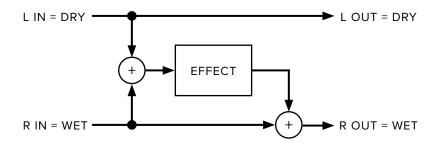
**ILLUMINE Only** — ILLUMINE is the only effect in the wet signal chain and will create a wet/dry output from a dry input. The mono/dry input is sent to the left output, and the wet signal is sent to the right output.
