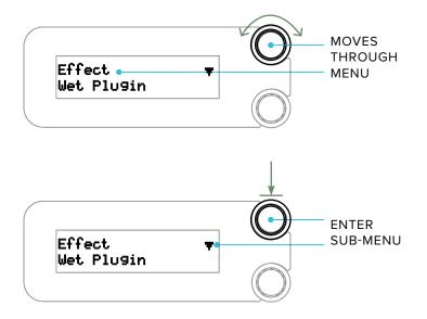
If  $\blacktriangle$  is displayed, pressing the top knob returns to the top-level menu. When the arrow is not displayed, pressing the top knob will jump to the **PRESET** screen.
