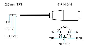
The MIDI INPUT is isolated and may be used in a daisy-chain connection.
