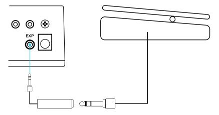
To connect a volume pedal, use a 3.5 mm to dual  $\frac{1}{4}$ " TS (stereo breakout) cable, such as a Hosa CMP-153. Connect as follows:
