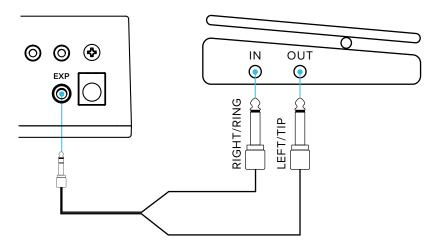
The volume pedal must be passive (unpowered).
