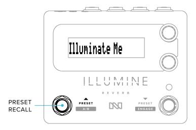
A long-press (>650 ms) of the left footswitch toggles between A and B parameter sets, if the A/B switch is selected as the Expression Input (see Expression Control Engine).
