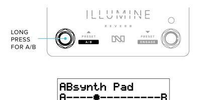
If the A/B Footswitch is long-pressed during a transition, the parameters will turn around and traverse a reverse path to the original state. If the A/B Footswitch is short-pressed during a transition, the parameters will jump to the destination state, effectively cancelling the transition period.
