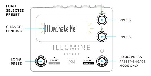
Since this option adds a secondary long-press function to the Preset footswitch, changes will occur upon switch release (see Actuation, p. 10).
