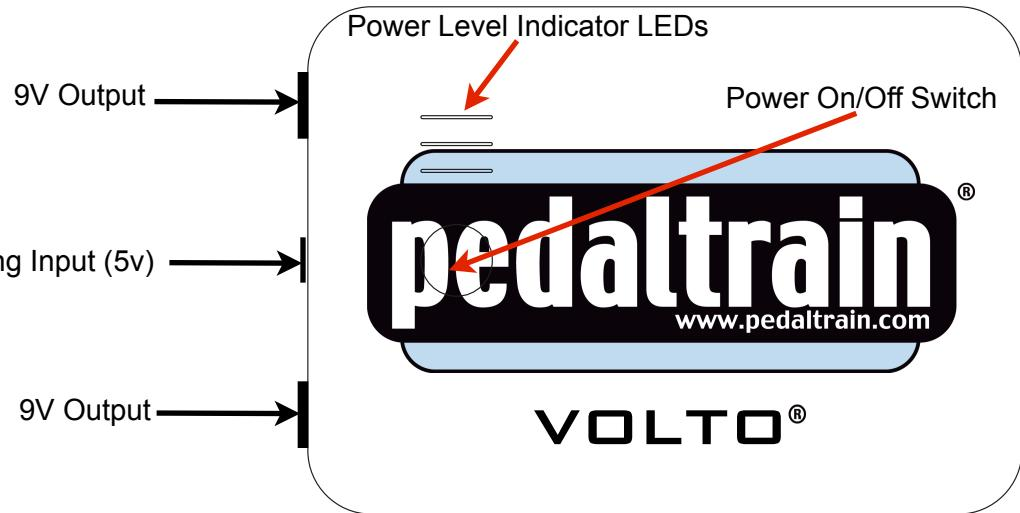
**Charging:** The first thing to do is make sure the VOLTO is fully charged. Use the supplied USB cable and 1.0A AC Charger with the appropriate adapter plug for your country. It takes an average of six hours to fully charge the unit from zero to full capacity. You can also recharge the VOLTO with any standard 5V output USB device such as a personal computer, a cell phone charger, or car charger. This is a high capacity battery, your results may vary depending on the charger used.
