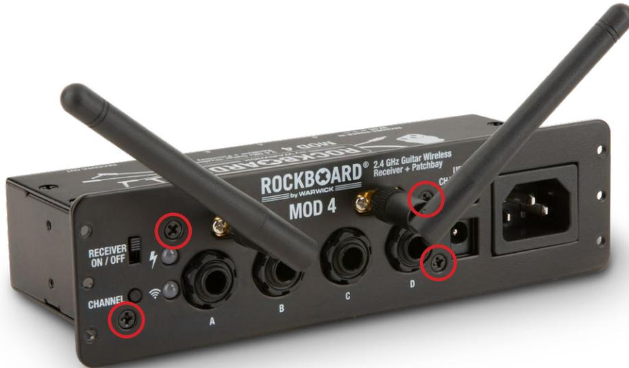
Remove the marked screws to release the front plate from your MOD using a PH2 Phillips head screw driver. The mounting nuts of the jack sockets do not have to be removed!
