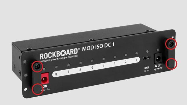
To mount the **RockBoard**<sup>®</sup> MOD ISO DC 1 on top or underneath your pedalboard, you must detach the front plate, so it will fit flush onto/under the board surface.
