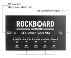
5 x switchable slots with 9V DC / 12V DC / 15V DC / 18V DC; Individual maximum output: 500 mA at 9V, 375 mA at 12V, 300 mA at 15V, 250 mA at 18V
