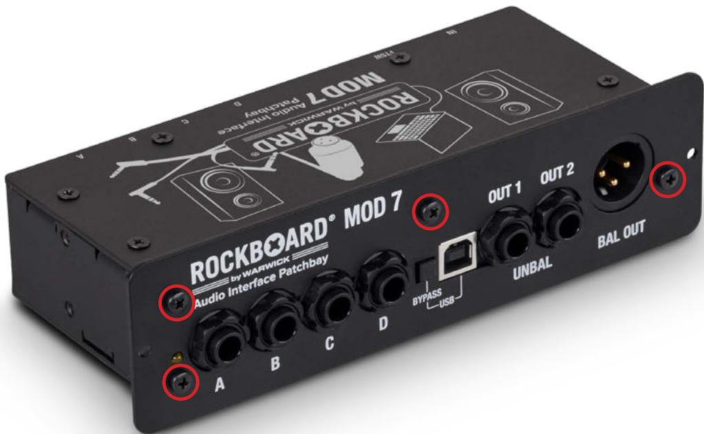
Remove the screws as indicated below to release the front plate from your MOD using a PH2 Phillips head screw driver. The mounting nuts of the jack sockets do not have to be removed!
