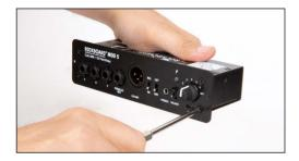
**STEP 1**Release the MOD's front plate by removing the screws indicated above.
