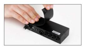
Apply self-adhesive hook tape or another reclosable fastener to the underside of the MOD housing.
