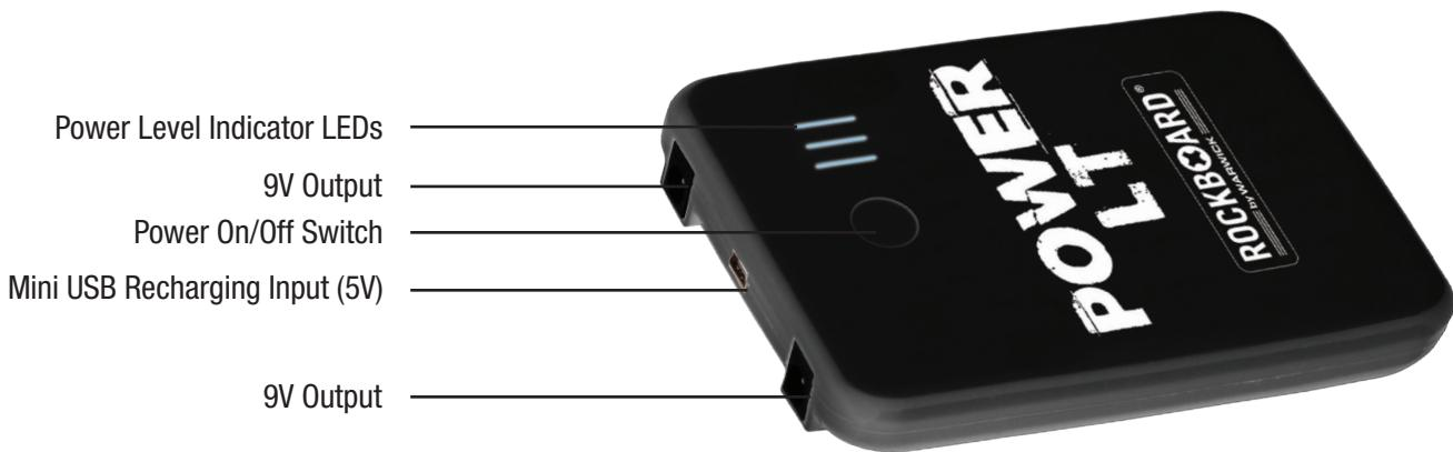
**Charging:** The RockBoard Power LT should be fully charged via supplied USB cable or power adapter with the correct plug for your country. Charging approximately takes 6 hours from 0 to full power. You can also charge the device via any standard 5V output USB device as e.g. personal computer, car hifi system, etc. Charging times always depend on battery health, battery power level and charger used.
