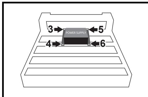
1. Insert screws (included with Voodoo Lab power supply) into RBO VKit 1 & 2 (on both sides) and use a Phillips screwdriver to attach to the power supply.
