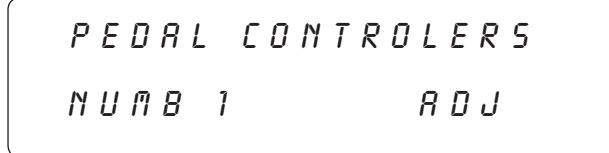
**Step 3** Use the PARAMETER ADJUST knob to select the controller to be assigned to the NUMB 1 parameter (either ADJ, IPED, IPSW or OFF).
