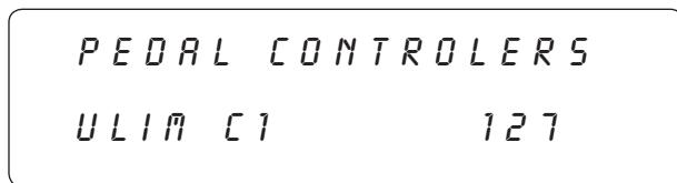
**Step 8** Turn the PARAMETER SELECT knob one step clockwise to access the Lower Limit parameter (for PARA 1).
