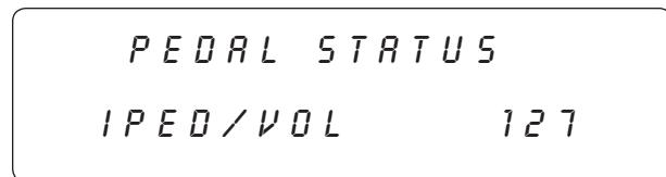
The IPED/VOL will only change in real time if the Internal pedal has been assigned to the IPED/VOL parameter. Otherwise to check pedal operation please view the parameter that it is assigned to. I.E.: If assigned to Chorus Rate got to the Chorus Function and look at the RATE parameter and move the pedal. You should see the value changing.
