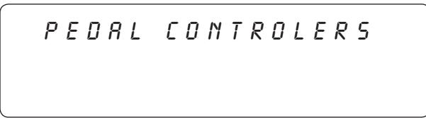
**Step 2** Turn the PARAMETER SELECT knob for the first parameter of the Controller Assign function. This parameter allows you to select a controller number for the NUMB 1 parameter to respond to.
