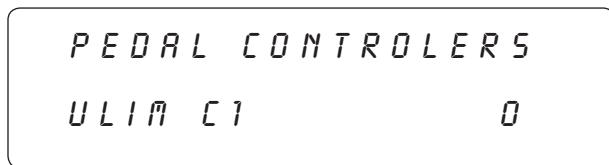
**Step 9** Use the PARAMETER ADJUST knob to select the lowest value which the parameter is not to fall below through when the heel of the expression pedal is down.
