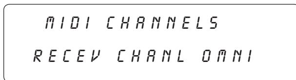
**Step 3** Turn PARAMETER ADJUST knob to select the appropriate Receive Channel 1-16, Omni and OFF
