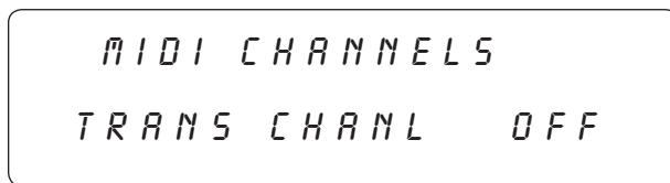
**Step 3** Turn PARAMETER ADJUST knob to select the appropriate MIDI Channel 1-16 and OFF.
