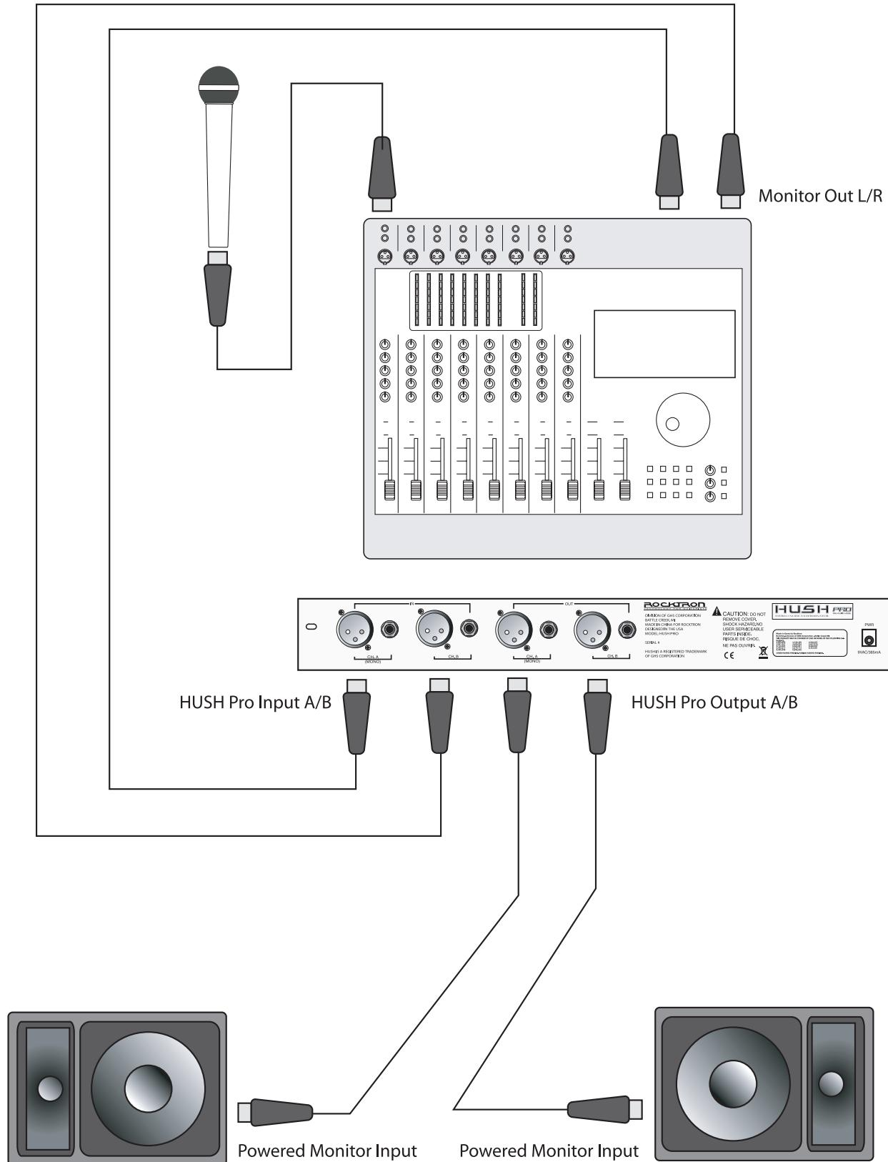
Connection direct mic plug into main input of channel. In this application the HUSH Pro acts as a "hard gate with noise reduction" which will help curb feedback. Can be used like this or with the HUSH Pro in the channel insert.
