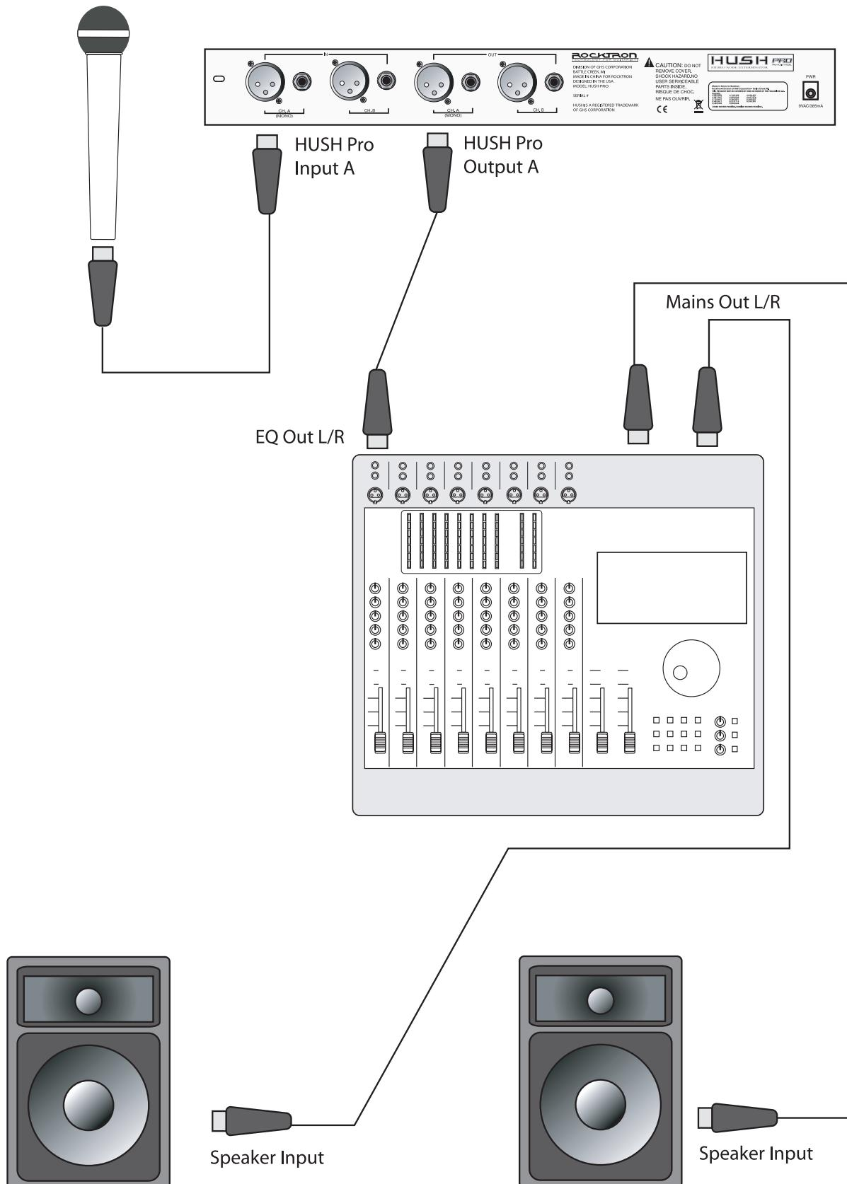
Connection powered box mixer to speakers using XLR jacks
