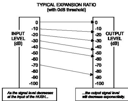
As the input signal drops further below the threshold point, downward expansion increases. A drop in the input level by 20dB would cause the output level to drop approximately 40dB (i.e., 20dB of gain reduction). In the absence of any input signal, the expander will reduce the gain so that the noise floor becomes inaudible.
