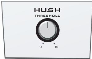
The front panel *HUSH Threshold* control determines the minimum input level at which the HUSH filter and downward expander will begin to operate. Setting this control too high will result in a loss of sustain, as notes will tend to die out much faster than they should. Conversely, when set too low, the expander will close too late (if at all) and the noise floor will remain audible.
