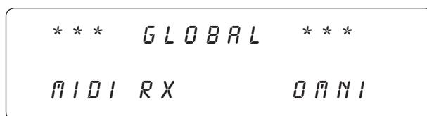
STEP 4 - To adjust the selected "PARAMETER", turn the HUSH THRESHOLD/PARAMETER ADJUST knob. The display will then show the adjusted parameter:
