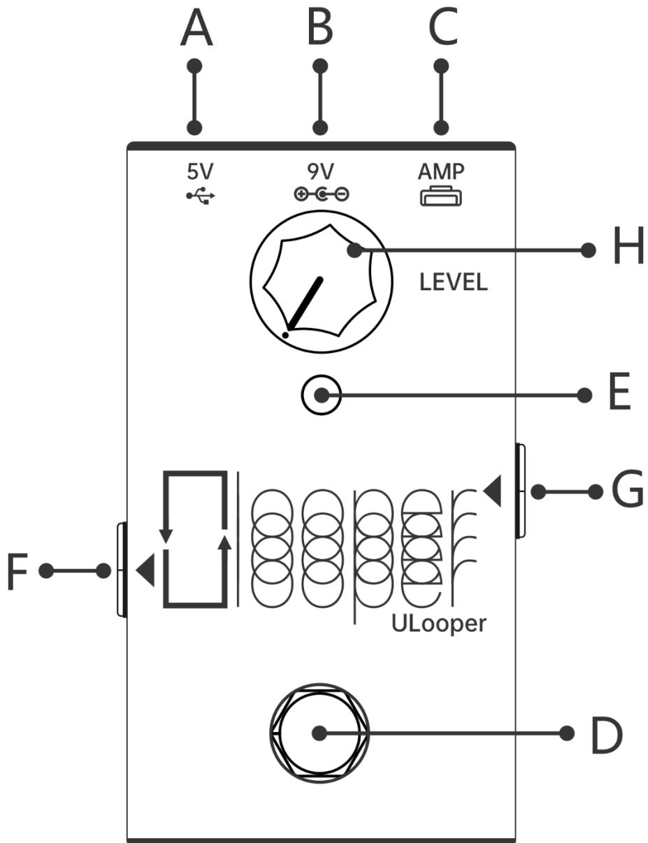
**A. 5V USB:** Connect to a power bank or phone charger. For firmware updates, connect to your computer via this port. This port requires a **minimum current of 1A**.
