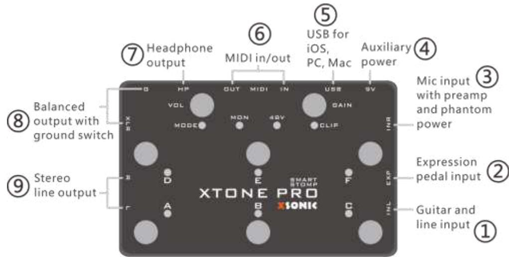
①**Guitar and line input:** Specialized input interface for guitar, bass, it is left channel. The interface does not pass any preamp, ensuring pure clear sound. This also means that the interface can be used for line input.
