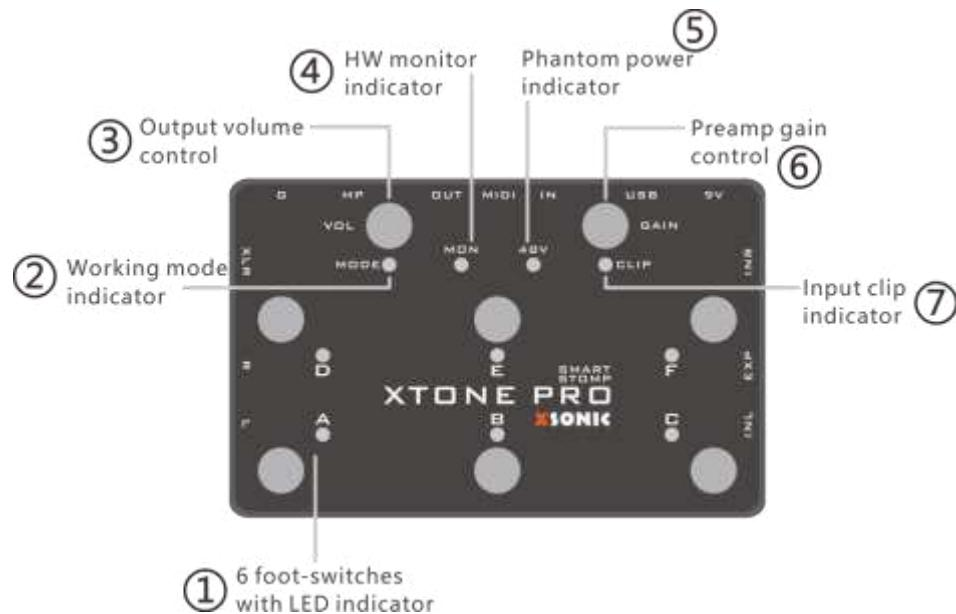
①**Smart foot switches:** 6 MIDI foot switches with LED indicator A, B, C, D, E, F; When the foot switch is pressed, the corresponding LED lights up and Pro sends MIDI commands outward. You can specify any features that you want to control via MIDI in software effects. For more details, please refer to the MIDI chapter below.
