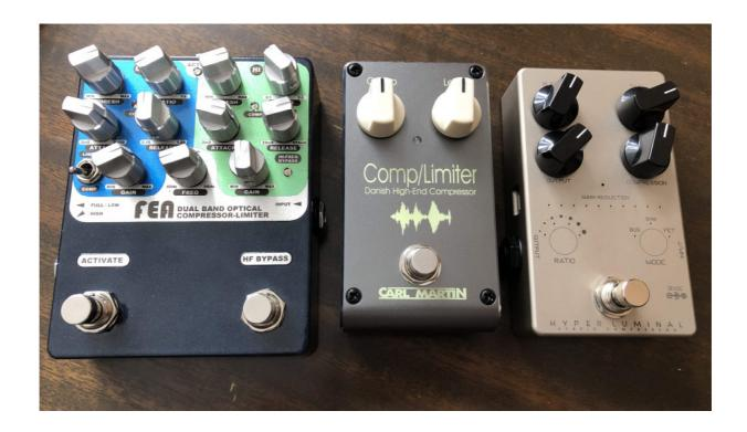
The foot switch is not true bypass. LED lights blue when engaged. There is no LED indicating threshold/gain reduction.
