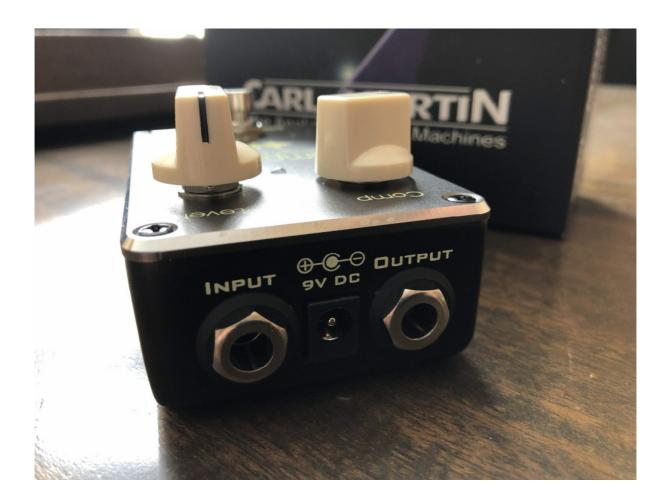
The enclosure is very attractive in my opinion. It is a nice anodized enclosure and with shiny bezel. It is quite light weight but seems well built. Top mounted jacks and 9-volt power input. The pedal requires 9 volts center negative pin and does not accept a 9-volt battery.
