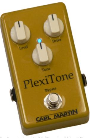
The Tone knob on the PlexiTone, is a high cut filter. With the knob set at full clockwise, you enjoy the full bandwidth of frequencies, so as you turn the knob counter clockwise, you start to filter out the high frequencies. This allows you to fine tune your tone regardless of which guitar/pickup you are using. You might find at high gain settings that reducing the highs will tighten up the sound, and at lower gain settings, the high frequencies will add some bite and crispness to your notes.
