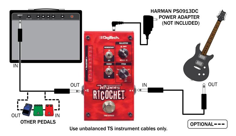
**NOTE:** The Whammy Ricochet should be the first pedal in your effects chain. Placing any effect in front of it may impact its pitch shifting performance.
