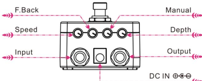
**Panel light ON/OFF:** Indicates effect or bypass status of Spark Flanger, when the panel lights up, the effect is on
