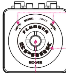
**Input/Output:** On the operating panel, regular triangle stands for "output" (▲). Inverted triangle stands for "input" (▼)
