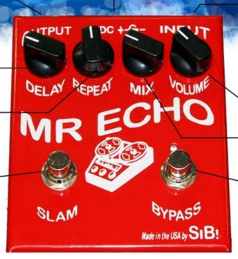
INPUT -- Plug your guitar or effect you plan on using in front of the MR ECHO in here. It works best towards the end of the effects chain. Plugging in here also turns the battery on Input impedance is over 1meg.
